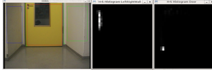
Fig. 7. Left: Areas which are considered for the ColorWallClassifier. Center: 2D hue-saturation histogram of the wall area. Right: 2D hue-saturation histogram of the door area.
