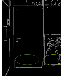
Fig. 8. Shows an image after Canny Edge detection. Green area: No texture in the bottom area of the door. Yellow area: Others objects have often textures in this area.
