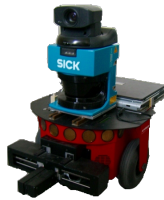
Fig. 1. Shows the mobile robot Pioneer2DX. It is equipped with a camera, a 2D laser range finder and an odometer.
