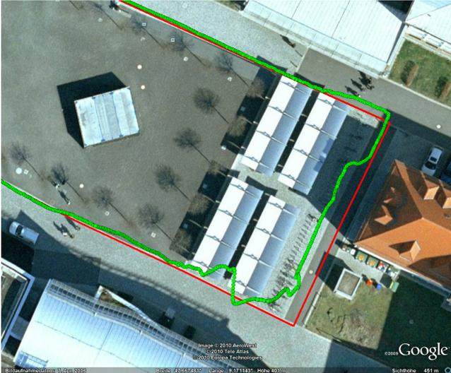
Fig. 5. Google Earth<sup>TM</sup> position plot of HTWG campus test.  $Q_t$  as random walk with horizontal  $\frac{\Delta\sigma^2}{\Delta t} = 1 \frac{m^2}{s}$  and vertical  $\frac{\Delta\sigma^2}{\Delta t} = 0.05 \frac{m^2}{s}$ . Red: estimated reference track; green: computed positions
