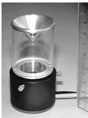
Figure 10: 360°-camera with conical mirror (scale in cm)
