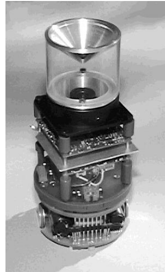
Figure 4: Khepera TM robot with camera module and custom made conical mirror, which permits sampling of the environment over 360^\circ , in a range of \pm 10^\circ about the horizon.
