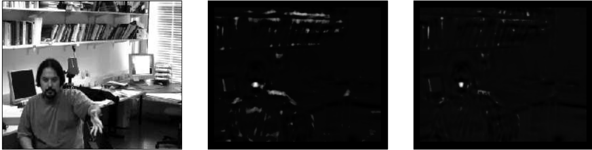
Figure 4.5: The effect of the bootstrapping procedure. In this figure we have plotted a test image (left) together with the support vector output before (middle) and after (right) bootstrapping. Bright pixels denote positions with large output values. After bootstrapping, the positive response on for example the bookshelf and the subject’s shoulder is damped by a noticeable amount.
