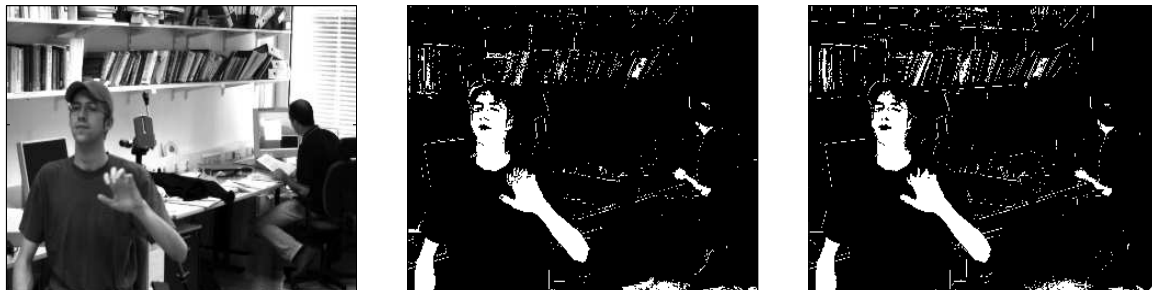
Figure 3.5: Support vector machines vs. neural networks in skin detection. The leftmost picture shows our test image. In the middle, we have the output of the SVM decision function, on the right we have the corresponding result from the neural network classifier. Note that both approaches lead to a very similar (visual) result, even though we expected the neural network solution to be slightly inferior.
