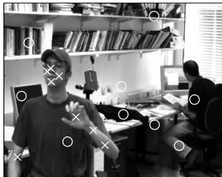
Figure 3.1: Data collection for training the skin color detector: This figure shows one of the 100 frames (out of 5197) from our video clips. The training samples are picked by hand and then stored automatically via a matlab program. The crosses/circles mark the skin/non-skin pixels that we collected from this image.
