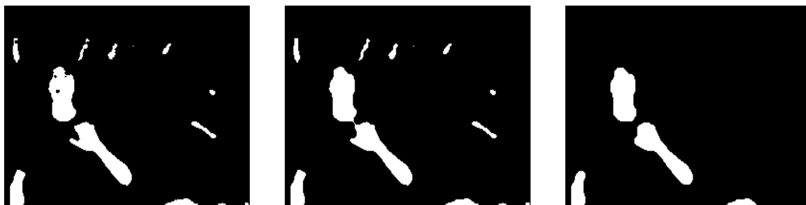
Figure 3.6: The three postprocessing stages. The left image shows the network classification output (Figure 3.5, rightmost image) after 5x5 median filtering. The subsequent closing transform yields the middle image. After re-opening the image, most of the unwanted skin pixels have been removed (right image).
